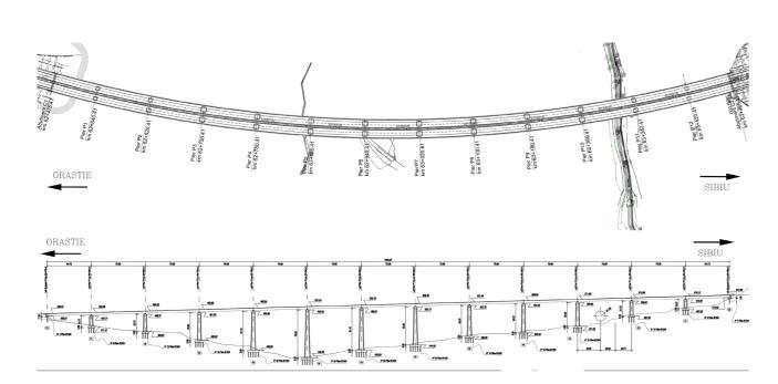
into the ground to offset the instability of the sandy soil of the valley. The viaduct was assembled in macro-segments in the assembly field on the ground with 80 tons gantry cranes and then incremental launched with the aid of a launching nose, proceeding simultaneously on each direction.
